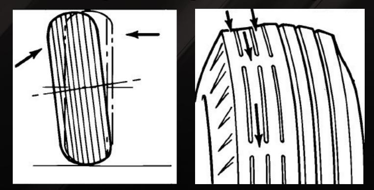
Wear on one side Excessive camber
