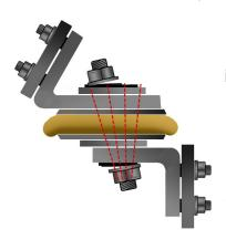
the material loses volume, becomes jelly-like and there is increased play in the motor mount bracketry. There may be noticeable load shifts as the motor is no longer firmly being held in place. Stress may begin to be felt by
