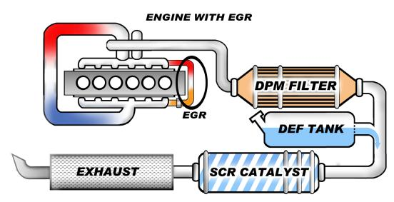
Under hood temperatures rise as the cooling system is over-burdened with the additional task of cooling the recirculating exhaust gas.
