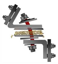
failure can end up causing the engine to sag or tilt to the point of making contact with the walls of the engine compartment.
