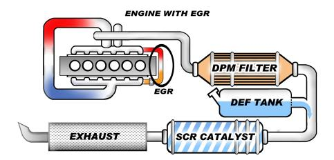
Under hood temperatures rise as the cooling system is over-burdened with the additional task of cooling the recirculating exhaust gas.
