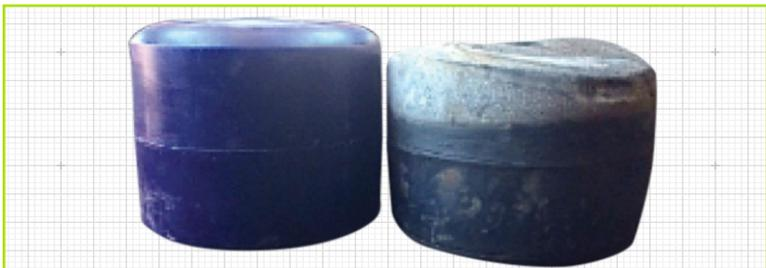
Load Springs subject to chemical attacks and should be replaced when worn. Otherwise ride height will be affected, causing numerous issues.
