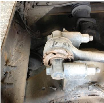
**Bushing Material Is Torn Or Cracked**
